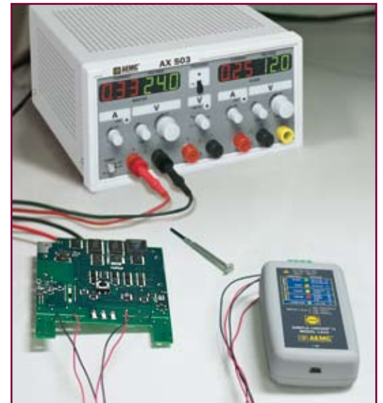
L432 recording two DC voltage supplies.
