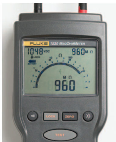
At 960 MΩ, this cable tests satisfactorily.
