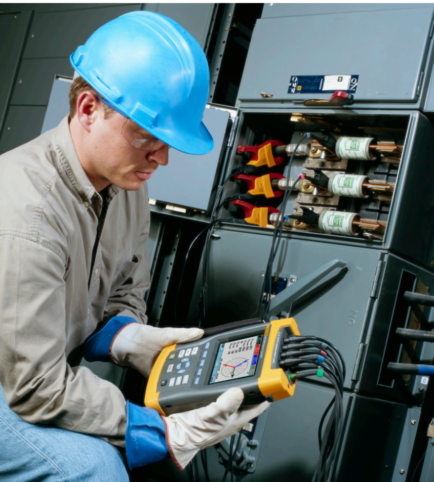
A three-phase power quality analyzer is an essential tool when conducting energy audits.
