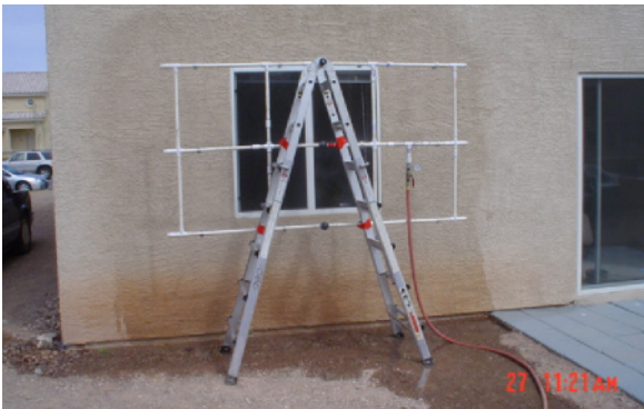
Calibrated spray rack used to simulate a rainshower.
